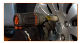
Lower the car and working in a cross order, tighten the wheel bolts. Use a torque wrench. Tighten it to 100 nm torque.
