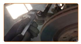
Loosen the lock nut securing the tie rod end to the tie rod. Use a combination spanner #21 (2 pieces).
