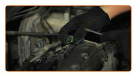
6 Unscrew the ignition coil bolts. Use a drive socket #8. Use a ratchet wrench.
