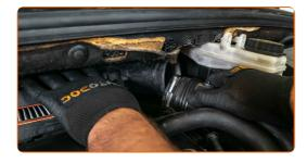
Tighten the clamp and fasteners on the air filter intake pipe. Use a combination spanner #7.
