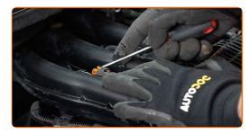
4 Unscrew the ignition coil bracket. Use a drive socket #8.
