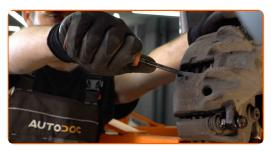
10 Remove the brake caliper.
