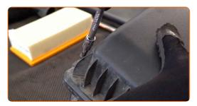
Reinstall the air filter housing.
