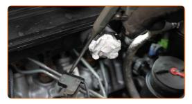
Unscrew the glow plugs. Use the spark plug socket #12. Use a torque wrench.
