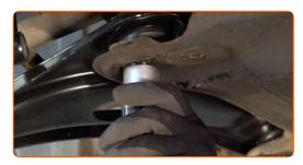
Tighten the front fastener connecting the control arm to the subframe. Use 12-point socket No.22. Use a torque wrench. Tighten it to 126 Nm torque.
