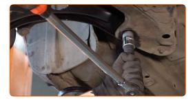
Tighten the ball joint fastener. Use a combination spanner #14. Use a drive socket #16. Use a torque wrench. Tighten it to 44 Nm torque.
