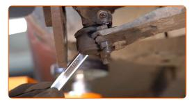
Remove the fastening bolt.
