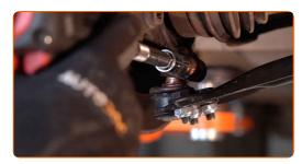
Screw the rear arm fastener. Use 12-point socket No.22.
