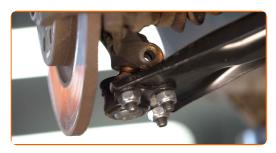
Install the fastening bolt. Use a hammer.
