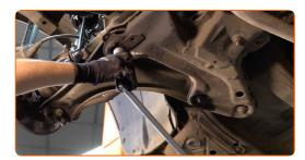
Unscrew the rear fastener connecting the control arm to the subframe. Use 12-point socket No.22. Use a tap wrench.
