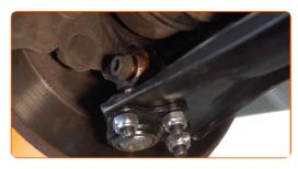
Screw the fasteners of the ball joint. Use a drive socket #16. Use a ratchet wrench.
