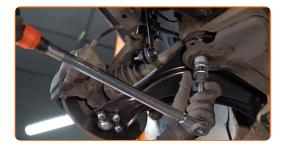
Tighten the rear fastener of the control arm. Use 12-point socket No.22. Use a torque wrench. Tighten it to 126 Nm torque.
