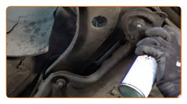
Unscrew the front arm fastener. Use 12-point socket No.22. Use a tap wrench.
