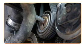
Pull aside the V-ribbed belt tensioner pulley. Use a 1/4" square drive extension bar. Use a ratchet wrench.
