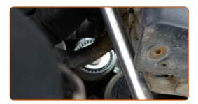
Turn the crankshaft pulley. This is necessary in order to make sure that the component operates properly. Use a drive socket #27. Use a ratchet wrench.
