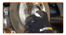
Unscrew the brake disc fastening. Use Torx T30. Use an impact screwdriver.
