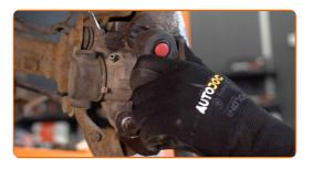
Remove the brake caliper.
