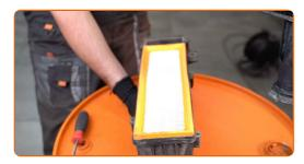
10 Remove the filter element from the filter housing.
