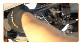
14 Remove the caliper bracket.
