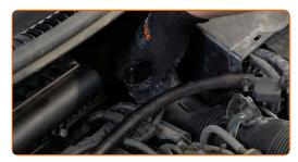
Remove the air intake pipe.
