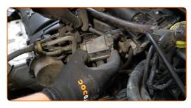
Detach the engine wiring harness connectors. Use a flat screwdriver.
