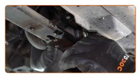
Attach the clamp of the lower coolant pipe. Use a combination spanner #7.
