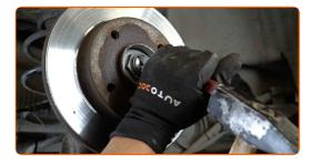
Unscrew the hub nut. Use a drive socket #36. Use a tap wrench.
