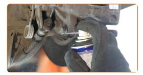
Unscrew the brake caliper fastening. Use a combination spanner #19. Use a drive socket #13. Use a ratchet wrench.
