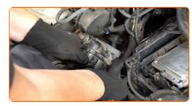
Clean the thermostat housing mounting seat. Use a seal scraper. Use all-purpose cleaning spray.
