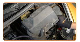
6 Unscrew the fasteners of the car battery terminals. Use a combination spanner #8.
