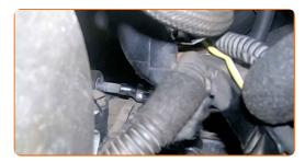
Detach the clip of the upper coolant hose. Use round-nose pliers.
