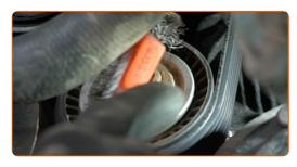
Loosen the tensioner pulley fastener. Use HEX No.H8. Use a ratchet wrench.
