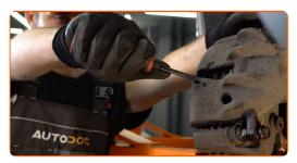
10 Remove the brake caliper.
