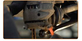
Unscrew the brake caliper fastening. Use a combination spanner #13. Use a combination spanner #15.
