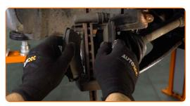
Replacement: brake pads – CITROËN C3 II Box Body / Hatchback (SC).
