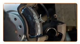
Replacement: brake pads – CITROËN C3 II Box Body / Hatchback (SC). Tip from AUTODOC experts:
