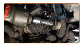
Unscrew the fastener connecting the stabilizer link to the shock strut. Use a drive socket #16.
