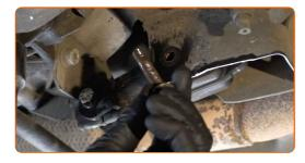
Unscrew the fastener connecting the engine mount to the gearbox housing. Use a drive socket #16. Use a ratchet wrench.
