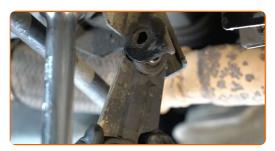
Replacement: engine mounts – CITROËN C3 I Hatchback (FC\_, FN\_).
