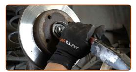
Unscrew the hub nut. Use a drive socket #36. Use a tap wrench.
