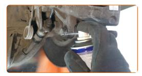
Unscrew the brake caliper fastening. Use a combination spanner #19. Use a drive socket #13. Use a ratchet wrench.
