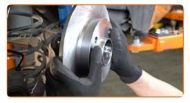
Tighten the wheel hub nut. Use a drive socket #36. Use a torque wrench. Tighten it to 270 nm torque.
