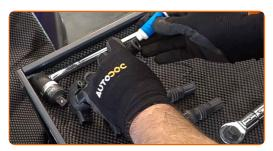
Screw new spark plugs and tighten them. Use the spark plug socket #16. Use a torque wrench. Tighten it to 22 nm torque.
