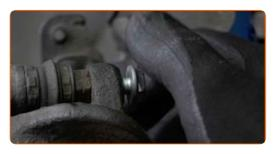
Tighten the brake caliper fasteners. Use a combination spanner #13. Use a combination spanner #15. Use a torque wrench. Tighten it to 27 nm torque.
