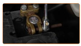
Disconnect the earth cable terminal from the battery.
