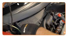
Screw in the fasteners of the cabin filter housing cover. Use a Phillips screwdriver.
