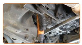
Support the gearbox. Use a hydraulic transmission jack.
