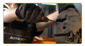
10 Remove the brake caliper.
