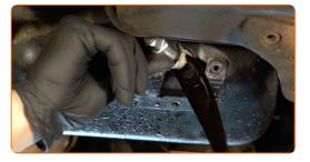
Replacement: engine oil and filter – CITROËN C2 Enterprise (JG\_). Tip from AUTODOC:
