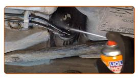
Remove the fuel lines from the car body.
