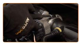
Disconnect the crankcase ventilation hose from the air duct.
