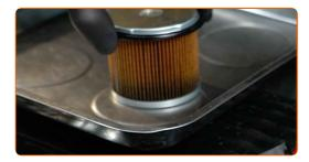
Pump the fuel out of the fuel filter housing. Use a hand-operated fluid syringe.
