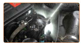
Unscrew the fasteners of the fuel filter cover. Use HEX No.H4. Use a ratchet wrench.
