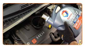
Replacement: engine oil and filter – CITROËN C15 Platform / Chassis (VDPD). Tip:
