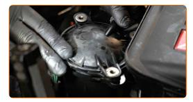
Tighten the fasteners of the fuel filter housing cover. Use HEX No.H4. Use a torque wrench. Tighten it to 9 Nm torque.
