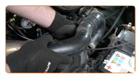
Screw the fastening clamp connecting the air duct to the air filter housing. Use a drive socket #7. Use a ratchet wrench.
