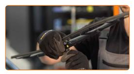
Remove the blade from the wiper arm.
