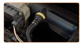
Install the crankcase ventilation hoses.
