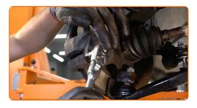
10 Remove the brake caliper.
