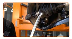
Remove the caliper bracket.
