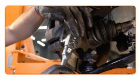
10 Remove the brake caliper.
