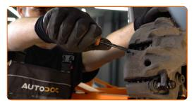
10 Remove the brake caliper.
