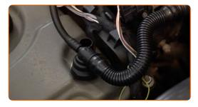
Remove the crankcase ventilation hoses.
