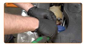
Remove the coolant reservoir cap.
