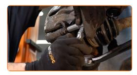
10 Remove the brake caliper.
