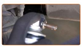
Install a new stabiliser link and tighten the fasteners. Use a drive socket #17. Use a ratchet wrench.
