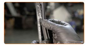
6 Remove the blade from the wiper arm.
