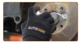
Unscrew the brake drum fastening. Use Torx T30. Use an impact screwdriver. Use a hammer.
