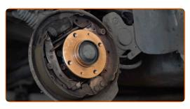
19 Install the brake drum and fasten it.
