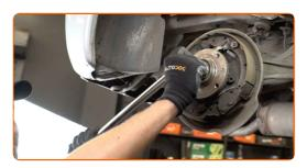
Remove the hub and the bearing together, since they are a sealed unit. Use 3-Arm Gear Puller.
