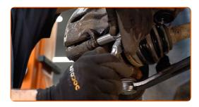
10 Remove the brake caliper.
