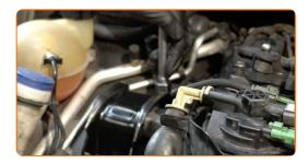
Tighten the fasteners that connect the engine mount to the car body. Use a drive socket #E14. Use a torque wrench. Tighten it to 60 nm torque.
