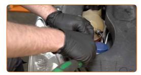
Remove the coolant reservoir cap.
