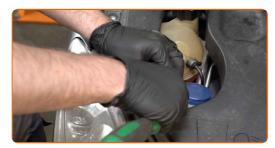
Remove the coolant reservoir cap.
