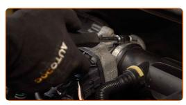
Disconnect the crankcase ventilation hose from the air duct.
