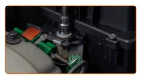
6 Remove the air filter housing.
