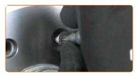
Tighten the brake drum fasteners. Use Torx T30. Use a torque wrench. Tighten it to 10 Nm torque.
