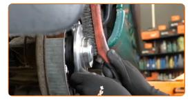
Treat the contacting surface. Use ceramic grease.
