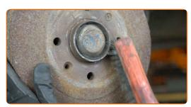
Unscrew the brake drum fasteners. Use Torx T30. Use an impact screwdriver.
