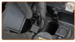
Take out the ignition coil from the spark plug well.
